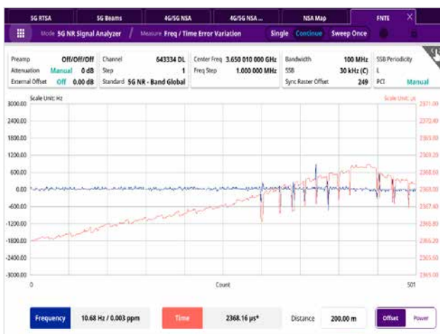
Figure 19 - Before and after timing and sync measurements using CA5G
